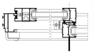
Horizontal cross-section of Topaze<sup>+</sup> straight design
